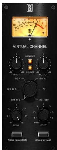
Figure 6: Virtual Channels; ›Brit 4k E‹ is the SSL 4000E, ›US A‹ is the API 1604, ›Brit N‹ is the Neve
